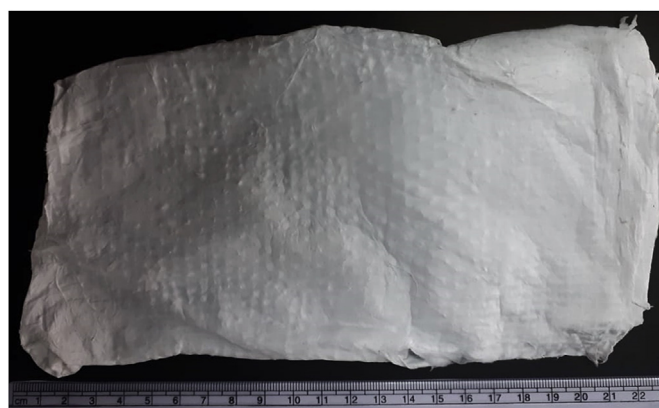
Fig. 15. PC nanofiber mat from 15 w/v% solution in 1:1 DCM-DMF mixture.
